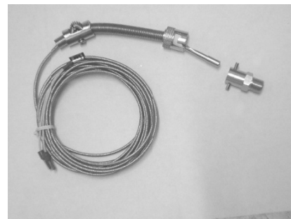
Gambar 7. Sensor suhu Thermokouple tipe-k.
