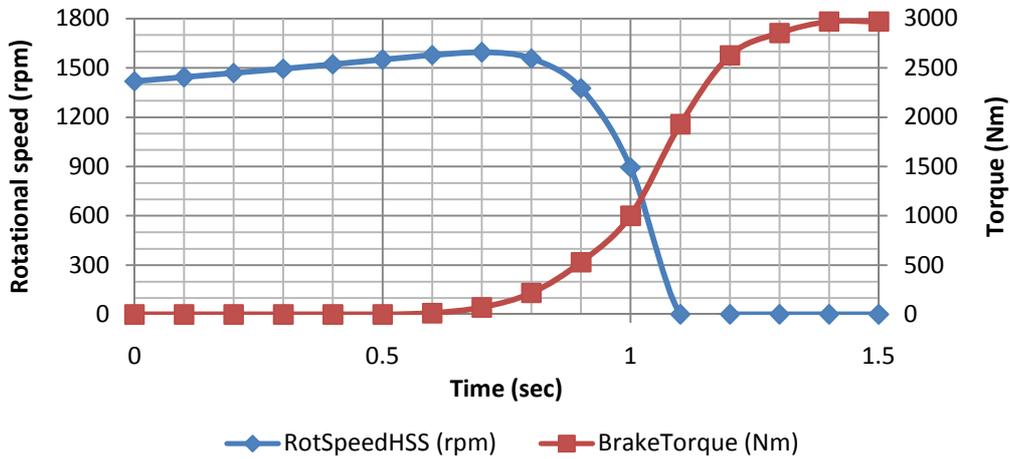
Figure 9: Simulation Result using the Real Turbine Parameters under Emergency Condition.
