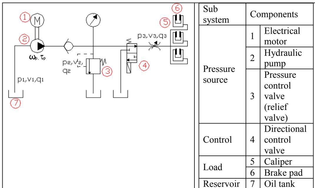
**Figure 3:** Design of Hydraulic System for Mechanical Brake.
