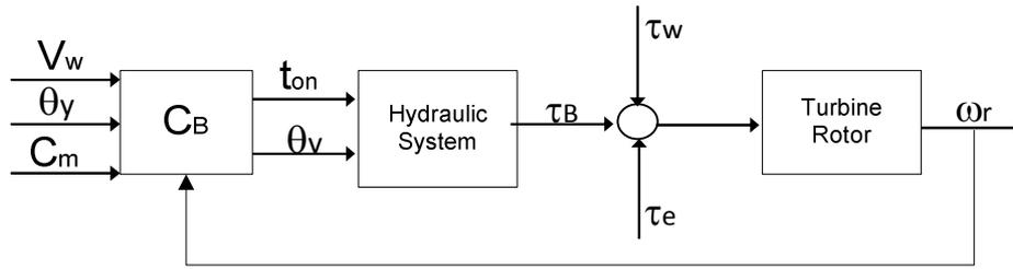
**Figure 4:** Block Diagram of the Hydraulic Brake Control System.
