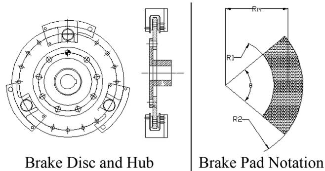
**Figure 2:** Design Of Brake Disc, Hub and Brake Pad
