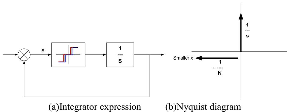
**Figure 4:** Illustration of the control system block diagram and its Nyquist diagram.
