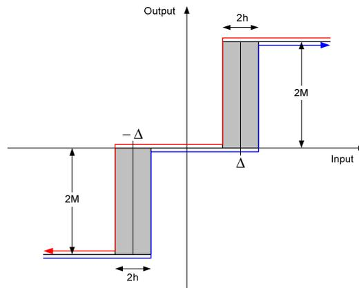
**Figure 2:** Input output characteristics curve (on/off control with dead band and hysteresis).
