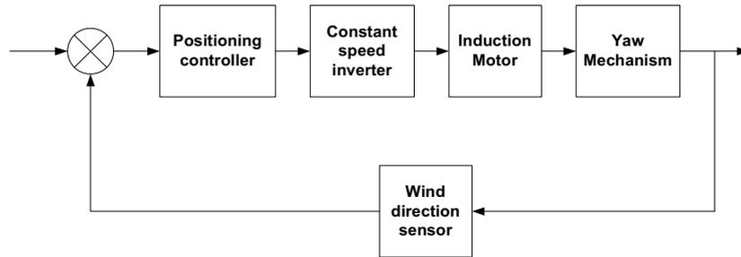
**Figure 3:** Block diagram of the yaw control system.
