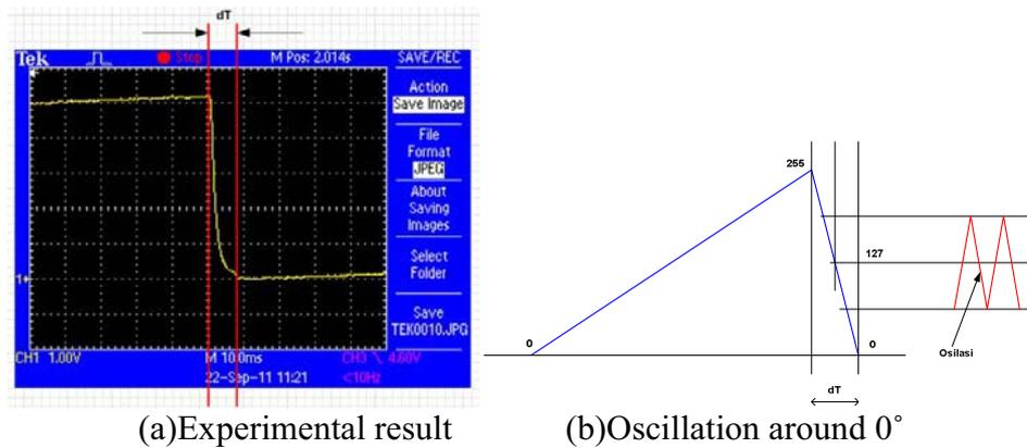
**Figure 6:** Wind direction sensor output and illustration of oscillation around  $0^\circ$ .
