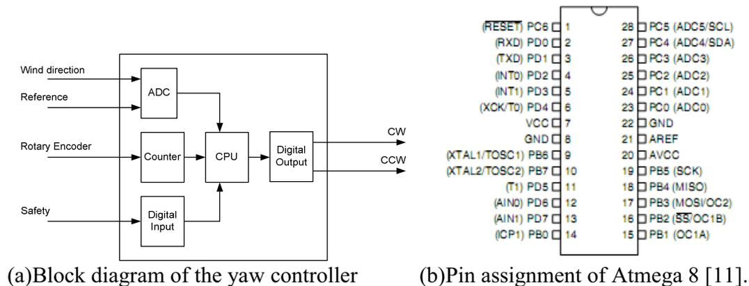
**Figure 7:** Realization of the yaw positioning electronic controller.
