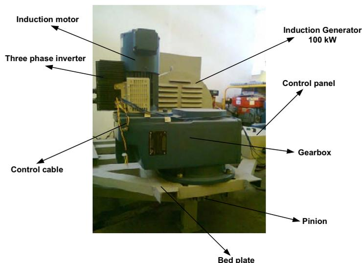
**Figure 1:** Yawing sistem set up in the laboratory.
