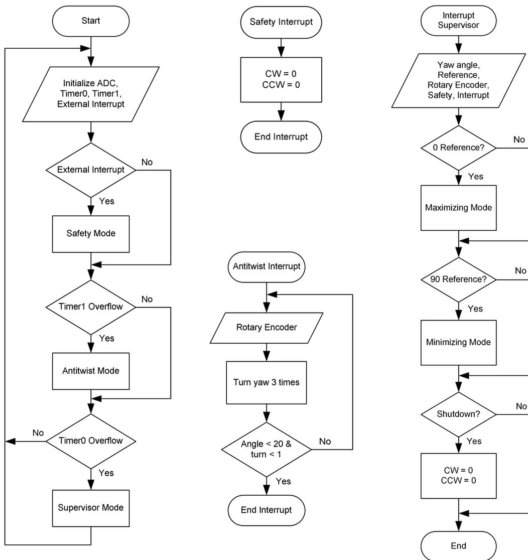
**Figure 8.** Flow chart of the control algorithm proposed in this paper.
