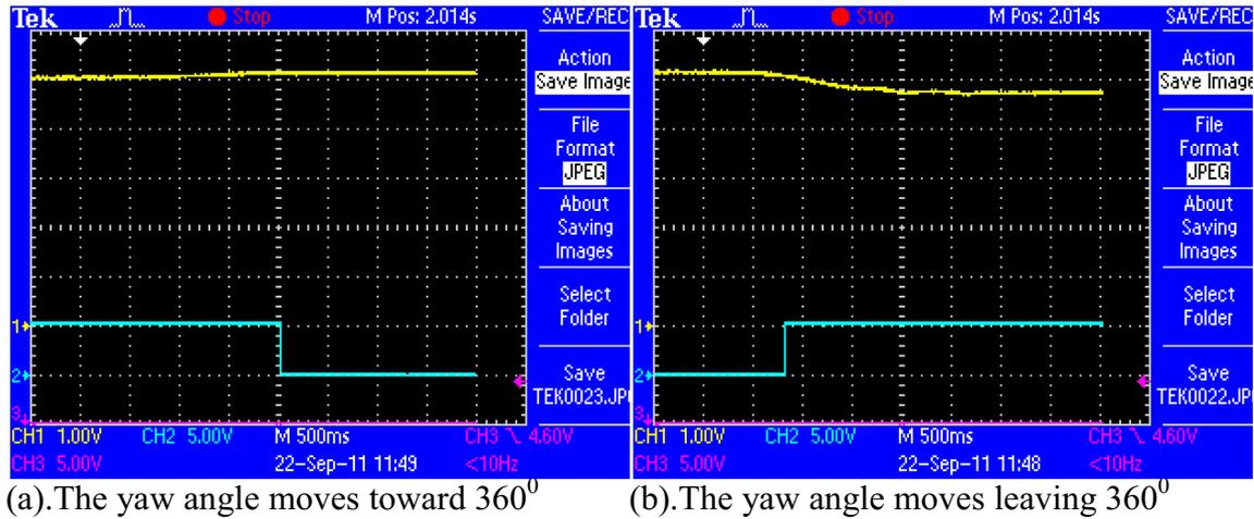
**Figure 11:** The yaw mechanism rotates in the CW direction at  $360^{\circ}$  vicinity.
