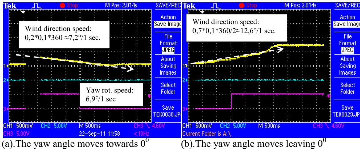
Figure 10: The yaw mechanism rotates in the CCW direction at  $0^{\circ}$  vicinity.
