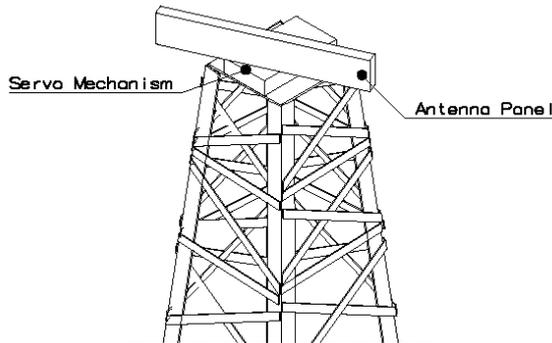
**Figure 2.** Illustration of the Antenna Structure.
