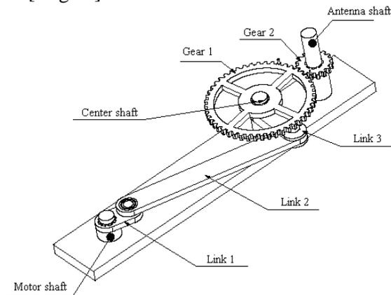
**Figure 3.** Shaking Mechanism for Micro-strip Array Antenna Used in a Surveillance Coastal Radar.
