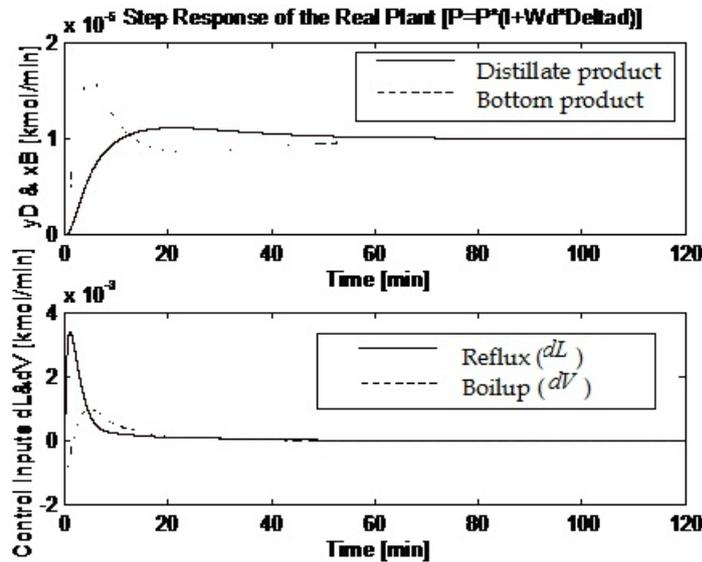
Figure 5: Step Response of Perturbed Real Plant Using  $K_\mu(s)$
