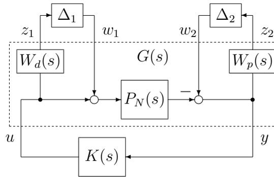
Figure 3: Generalized Plant for  $\mu$  Synthesis
