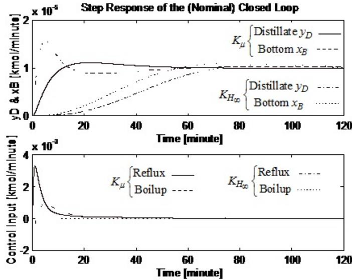
Figure 4: Nominal Step Responses Using  $K_\mu(s)$  and  $K_{H_\infty}$
